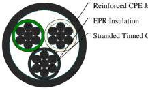
Reinforced CPE Jacket Stranded Tinned Copper Conductor
